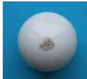
Figure 10: 5 Spark roots after 50 breakdowns on an electrode with 300 \mu\text{m} coating thickness.
