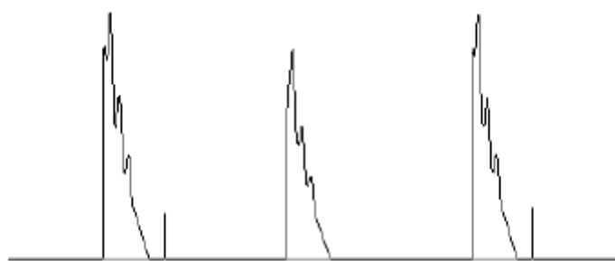
Fig. 12. Current flow from Phase A Winding to C_0 through D1
