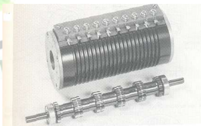
Fig.12.. Stator and rotor of a five-stack VR motor. (Courtesy of MINEBEA Co. Ltd.)
