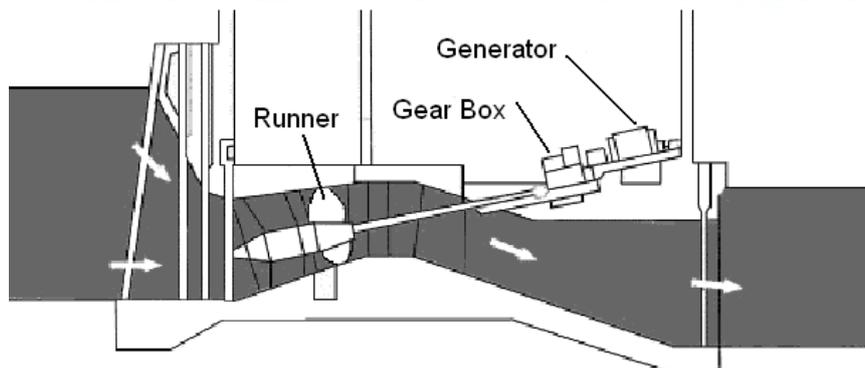
Figure 5 Tubular Turbine
