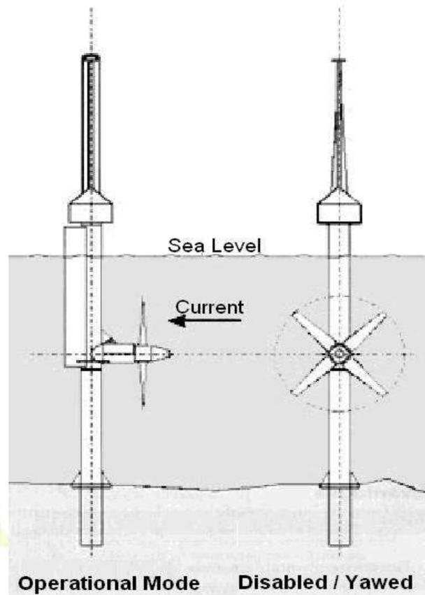
Figure 7 Schematic of an axial flow, seabed mounted marine current turbine
