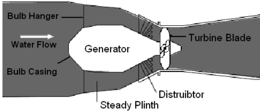
Figure 3 Bulb Turbine
