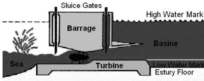
Figure 2 Ebb generating system with a bulb turbine
